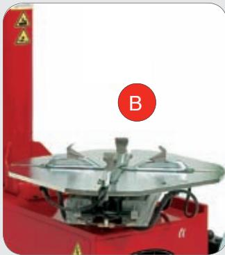
**EN** **SELF-CENTERING TURNTABLE:** System able to lock rims from 11" to 27" without adapters and adjustments. It employs unique rod geometry to ensure constant and even clamping power throughout all rim diameters. Available special optional adapters UWA24 and UMA for extended clamping capacity from 6" to 32".
